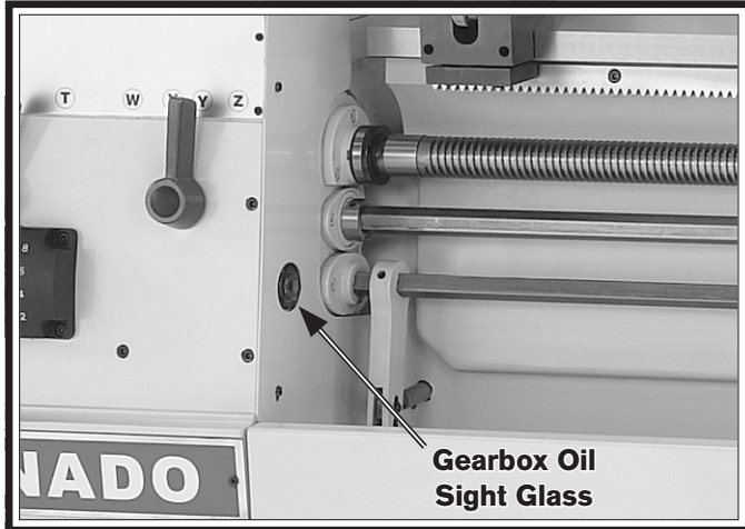
Figure 102. Location of quick-change gearbox oil sight glass.
